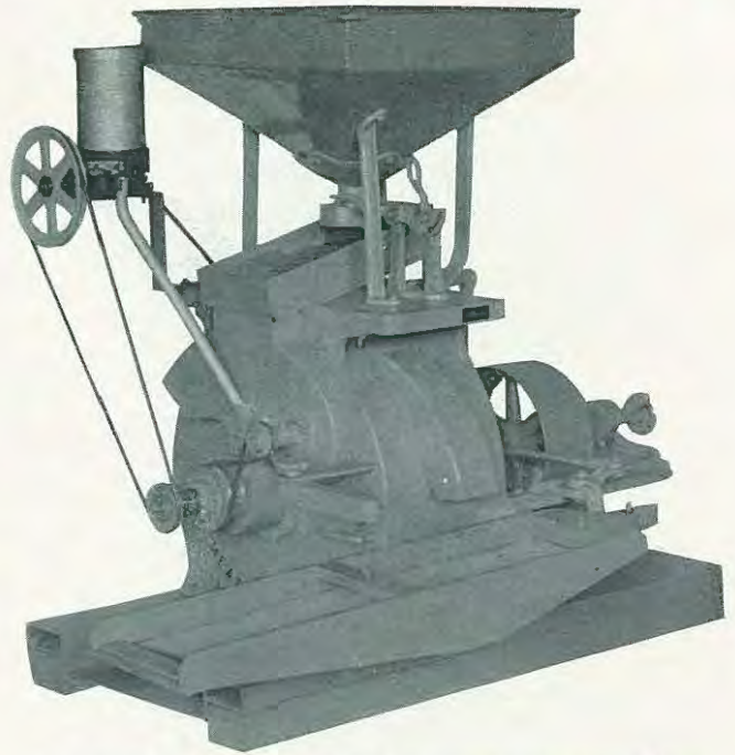
Showing 24" MEALMASTER equipped with open Sifter and Enrichment Feeder.
